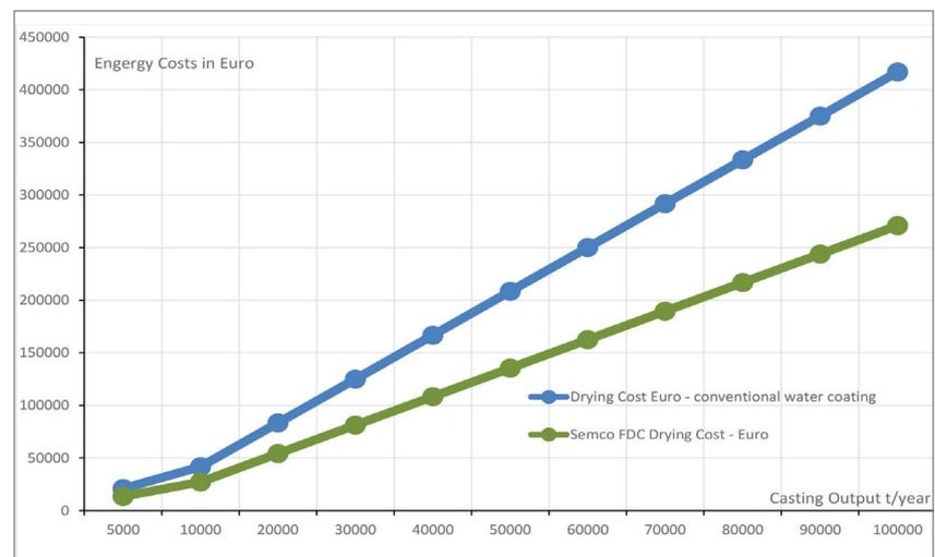
Figure 1. Approximate coating drying costs per annum versus casting output
